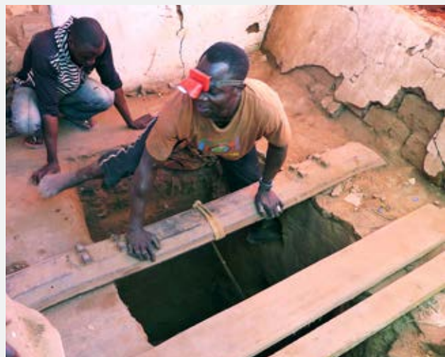
Miners climb out of a mine shaft by placing their hands and feet in holes carved out of the sides of the pit shaft. They use a rope attached to a beam stretched over the mouth of the pit as support. Sometimes the rope cuts and miners fall, a miner told researchers, May 2015 © Amnesty International and Afreewatch
